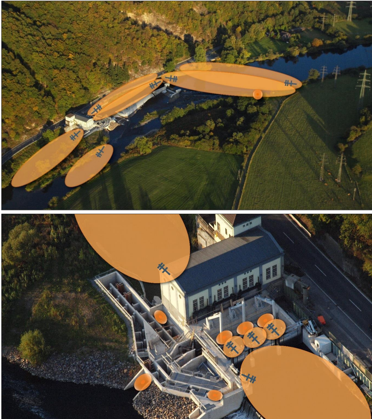
Figure 3.3. Overview of radio antennas and their approximate detection ranges used to record signals from radio tagged smolts at Unkelmühle power station. Upper panel: Overview of the power station area. Lower panel: Power station area in more detail. Detection ranges with antenna symbols indicate the use of aerial Yagi antennas, whereas ranges without antenna symbols indicate the use of underwater coaxial antennas Photos: Wikimedia Commons.
