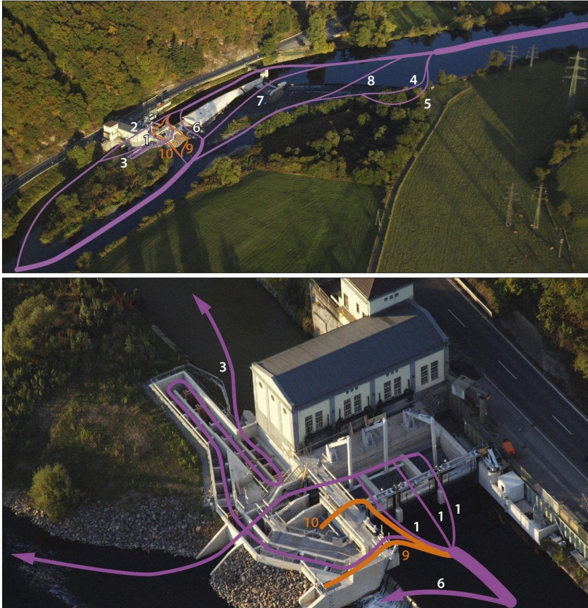
Figure 2.2. The different routes downstream migrating fish can use to pass the Unkelmühle power station: 1) via the surface bypass; custom-made openings in the racks that leads fish to a route outside the turbines via the flushing channel, 2) through turbines if they slip through the bar spacing of the racks, 3) through the vertical slot fishway constructed for upstream migrants, 4) through the nature-like fishway, 5) through the canoe pass, 6) via the ice gate, 7) over the spillway gate, 8) over the dam, 9) via the bottom bypass for eel, and 10) via side bypasses for eel (the two latter, indicated in orange, are only in operation during the eel run in the autumn). Numbers in both panels refer to the different migration routes. Photos: Wikimedia Commons.
