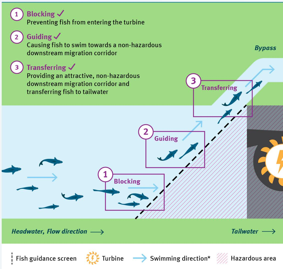
Schema (top view) of the three functions of a fish protection system: blocking, guiding, transferring.
