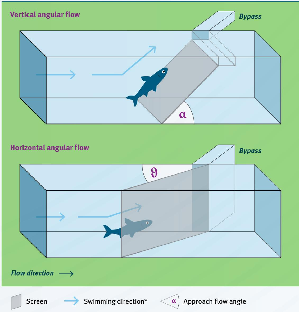
Fish protection screens with vertical angular flow have a guiding effect towards the surface and guide the fish to the bypass close to the surface. Fish protection screens with horizontal angular flow have a lateral guiding effect towards the bypass. The approach flow angles of the screens have a decisive influence on their guiding function (horizontal approach flow angle  $\vartheta$ , vertical approach flow angle  $\alpha$ ).
