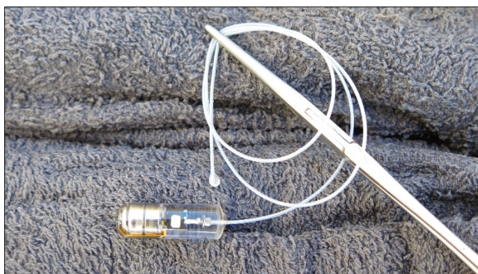
Figure 2.2. The eels were tagged with small radio transmitters (dimensions 9 x 30 mm; mass in air 4.3 g). Photos by Eva B. Thorstad.
