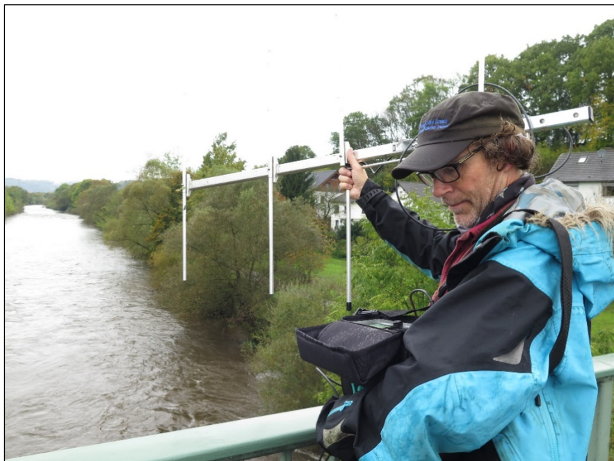
Figure 2.8. Tagged fish were also positioned by manual tracking, by walking along the river or using a bike or boat searching for tagged fish with a portable antenna and receiver. Searches for tags from fish were also done in cormorant colonies. Photo from the Sieg by Eva B. Thorstad.
