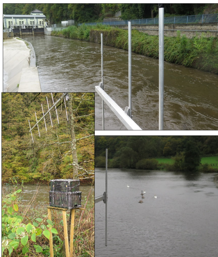
Figure 2.6. Downstream migration of tagged fish was studied by using stationary receivers, which automatically stored information on time and identity of tagged fish when they were within the detection range of receiver antennas. Photos from the Sieg by Eva B. Thorstad.
