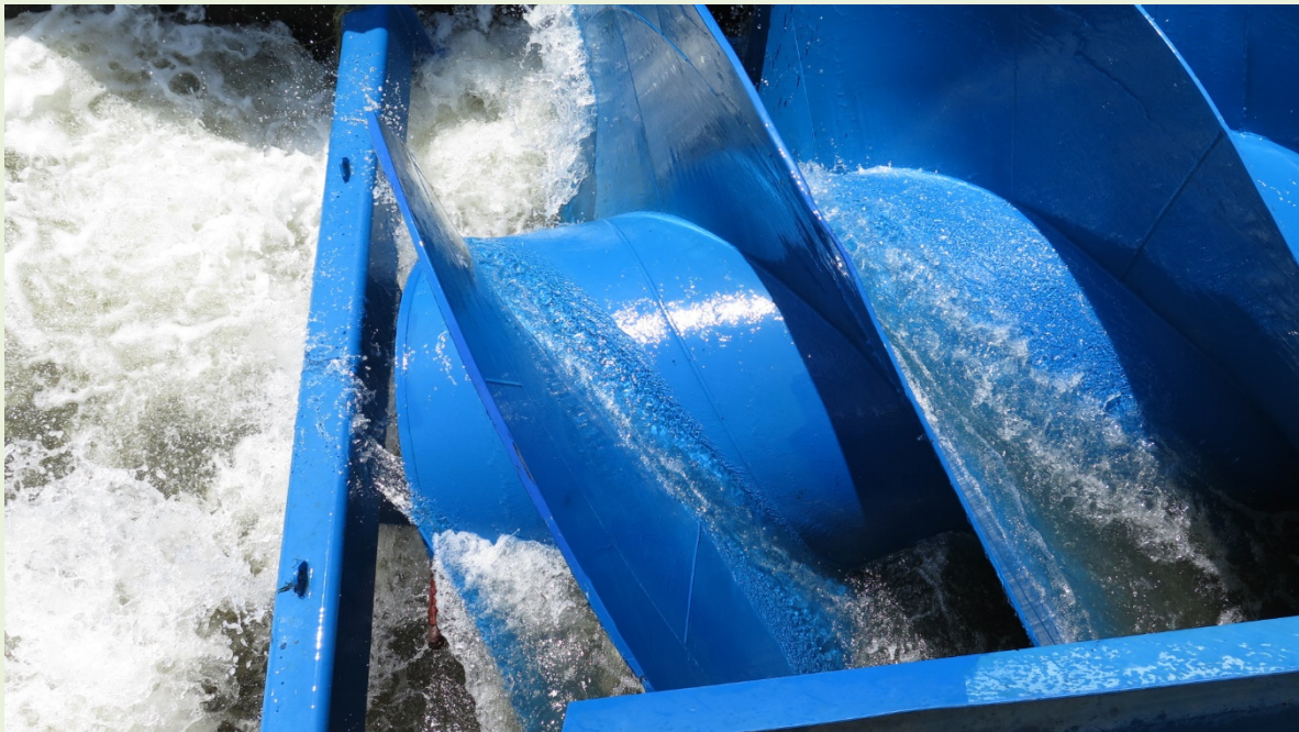
Lower end of the Archimedes screw at the Kuhlemühle power station in the Diemel. Photo by Eva B. Thorstad.
