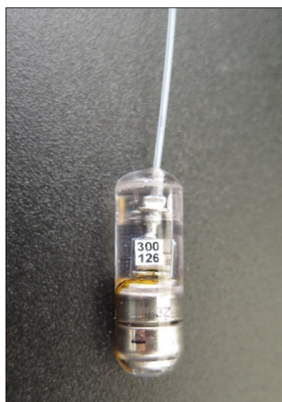
Figure 2.2. The eels were tagged with small radio transmitters (dimensions 9 x 30 mm; mass in air 4.3 g). Photos by Eva B. Thorstad.
